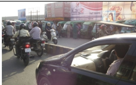
3. On-street parking on both sides of the road narrowing the effective carriageway width
