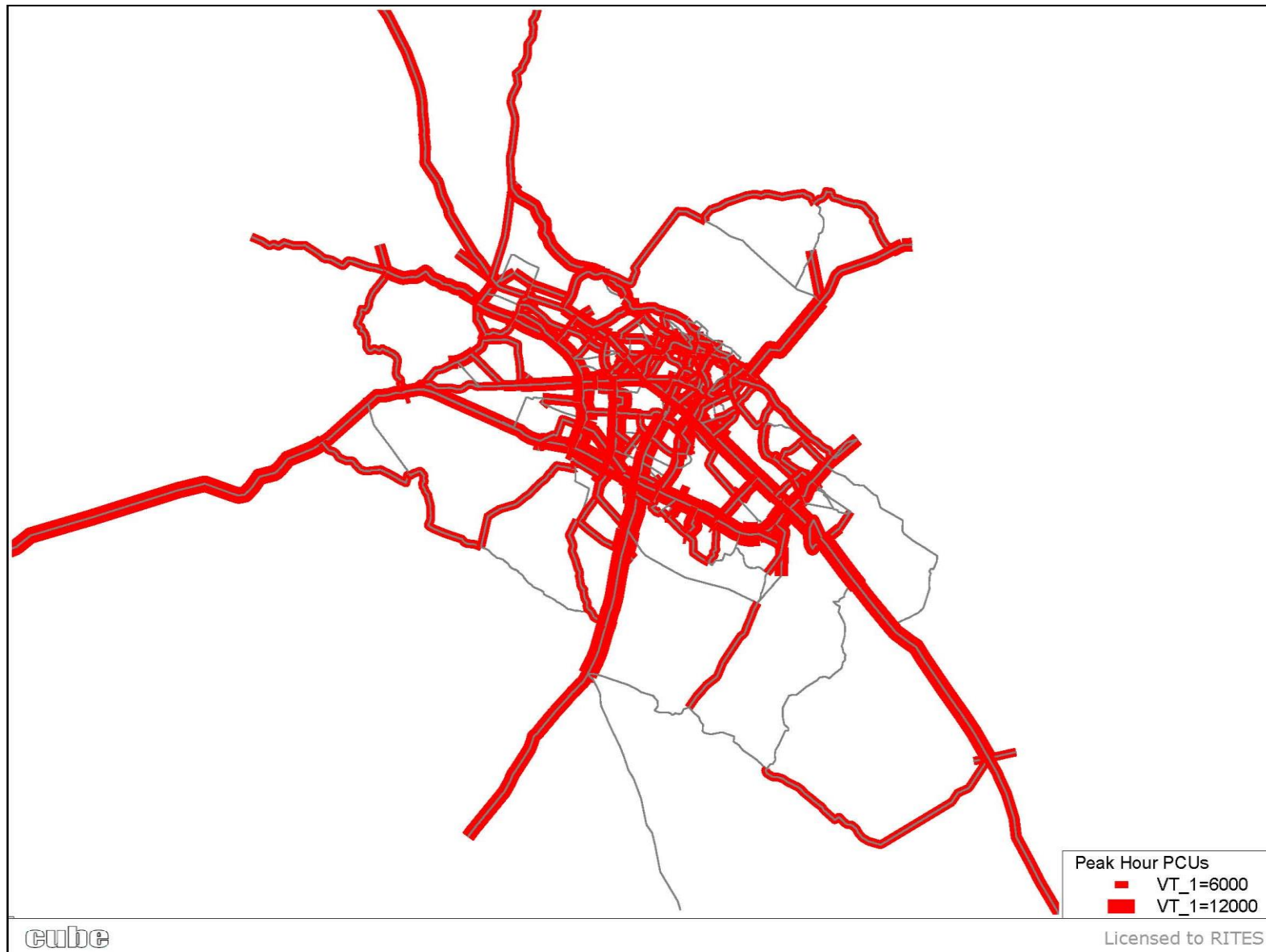
FIGURE 3.28: TRAFFIC ASSIGNMENT FOR PEAK HOUR TRAFFIC (IN PCU'S) ON ROAD NETWORK IN BAU SCENARIO 2041
