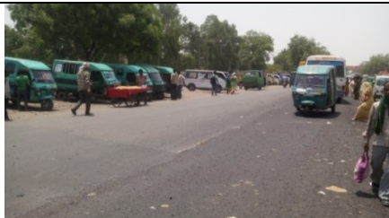
3. On-street parking on both sides of the road reducing the effective carriageway width.
