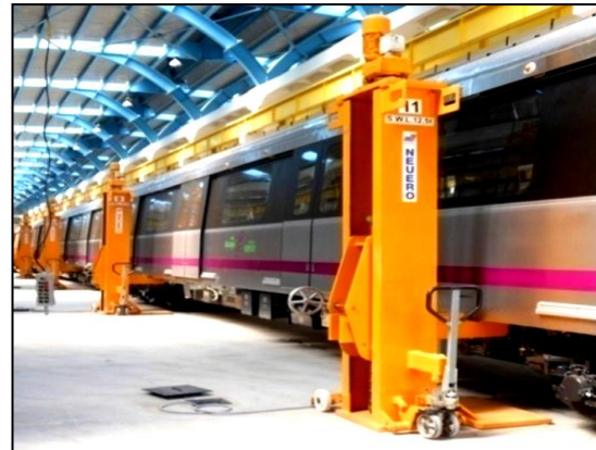
Synchronized Pit Jacks
