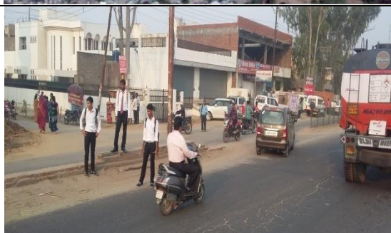
1. Lack of pedestrian facilities like footpath and FOB results in pedestrian spillover on road.
