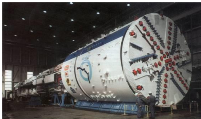
FIGURE 5.27: EARTH PRESSURE BALANCE TBM
