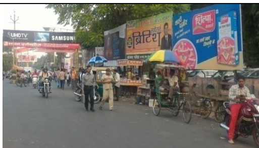
3. Encroachments along carriageway reduces effective road width.
