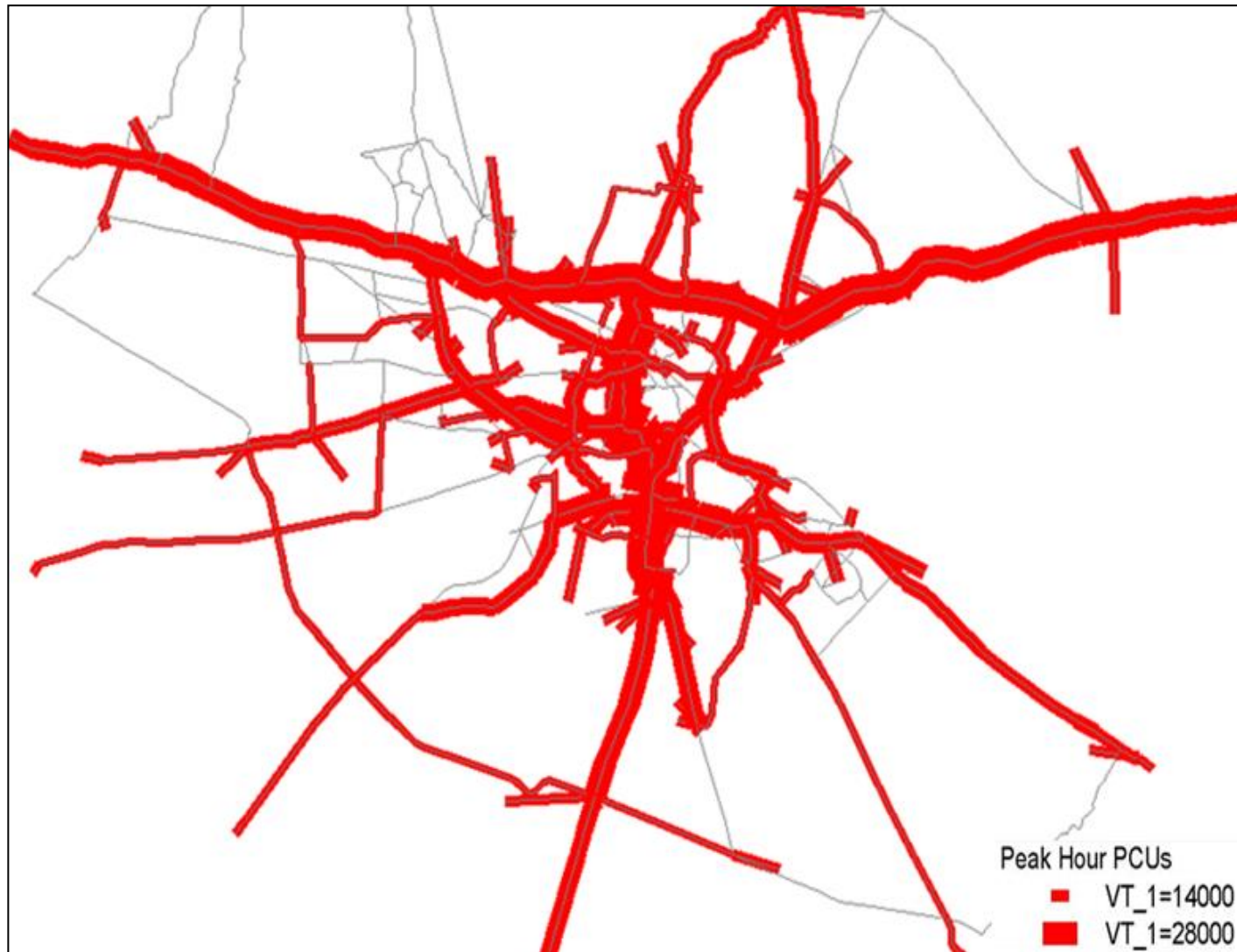
FIGURE 3.27: TRAFFIC ASSIGNMENT FOR PEAK HOUR TRAFFIC (IN PCU'S) ON ROAD NETWORK IN BAU SCENARIO 2041
