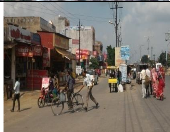
2. Heavy Encroachment leads to loss of carriageway width
