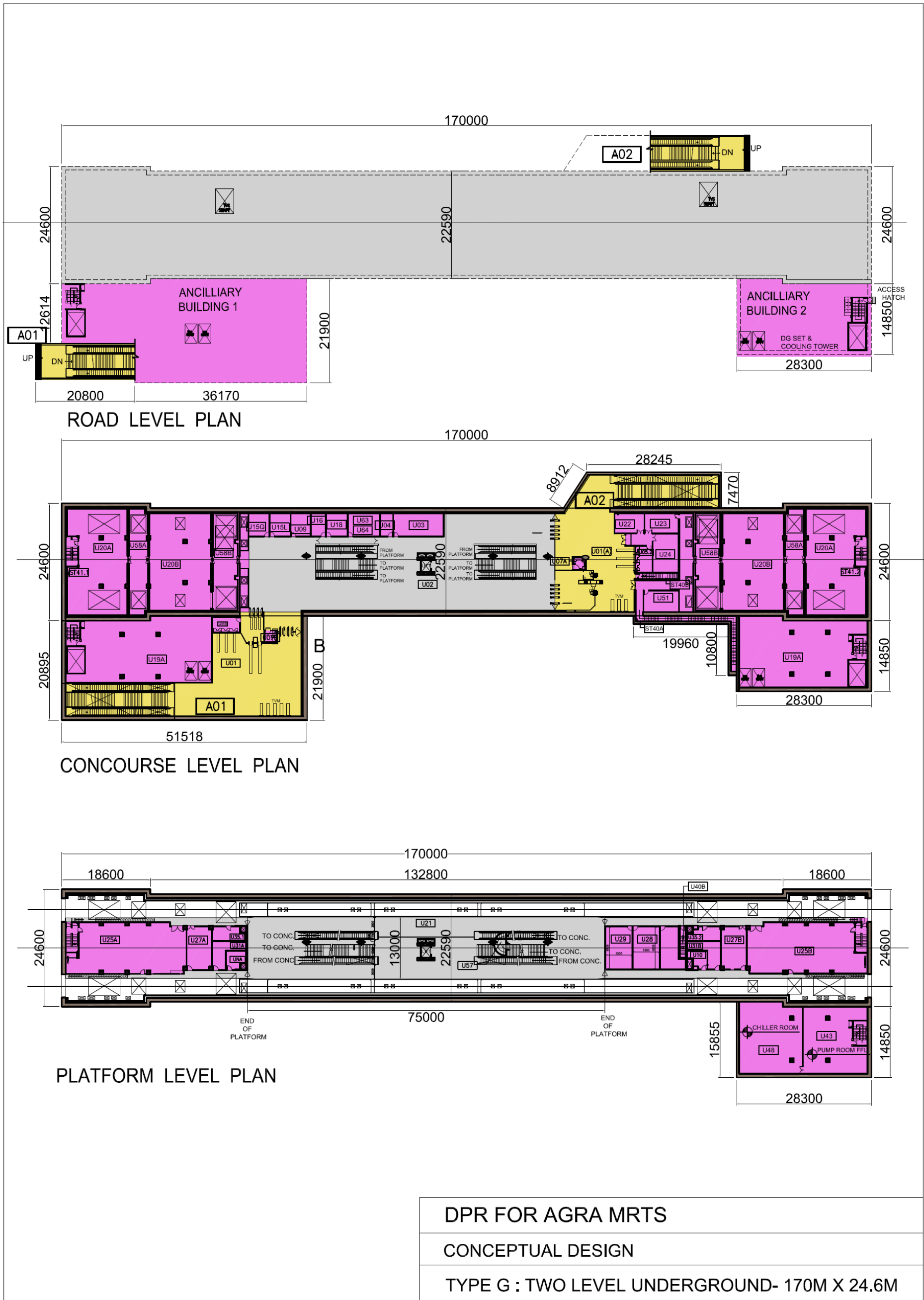
FIGURE 6.10: TWO LEVELS UNDERGROUND STATION – TYPE G
